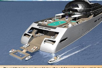
The yacht's tenders are stowed below aft in a full-beam tender bay, which also accommodates a submarine, speed boats, jet skis, crafts, ribs and all equipment for diving, snorkelling, and other water sports.
